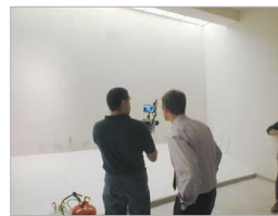
Infrared QA of foamed-in-place insulation behind 1" plaster – effective year-round (240F)
